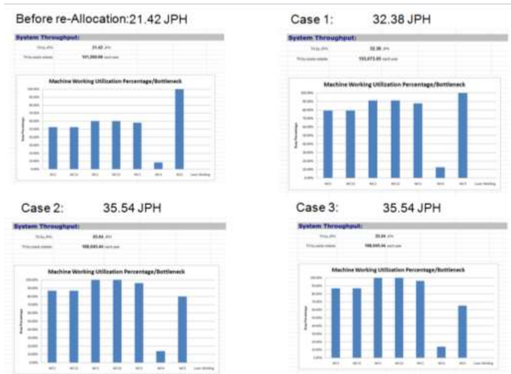
Figure 5-17 Throughput results when control procedure is changed
