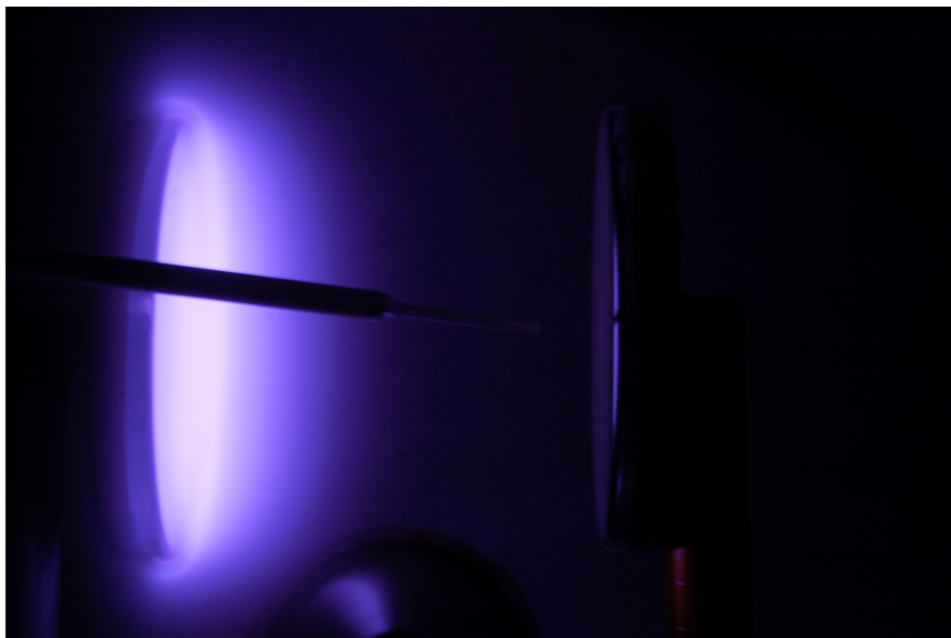
Figure 3.11: The glow discharge operating on argon at 350 mT and 40 mA. A planar Langmuir probe partially blocks the cathode on the left.
