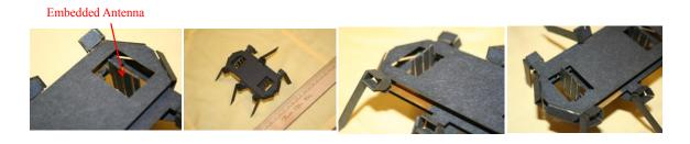
Figure 3.21: Embedded antenna inside a crawler robot.
