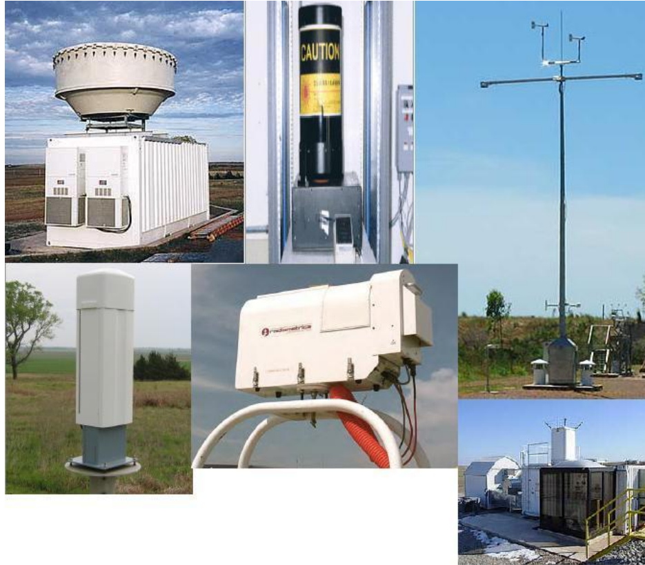
Figure 10: Some of the instrumentation at the ARM site: From left to right is the Millimeter wave cloud radar (MMCR), Micropulse Lidar (MPL), Surface Meteorological Instruments (SMET), Vaisala Ceilometer (VCEIL), Raman Lidar (RL)
