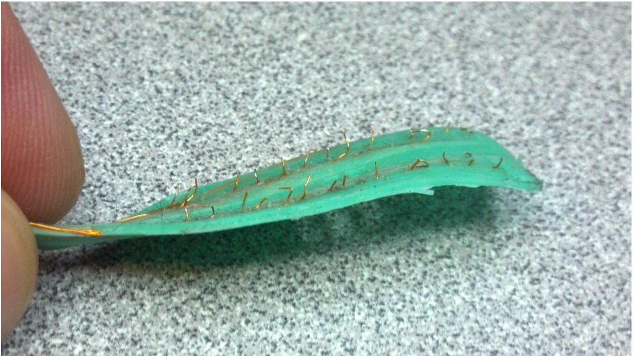
Figure 17: Side view of the prototype electrode plate.
