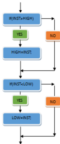
Figure 20: Finding the Highest and Lowest rates using two 'if' loops.
