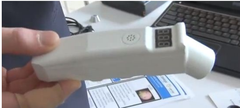
Figure 3: BabyBeats prototype as of 13 June 2012. Note that there is only one numerical readout - this outputs the fetal heart rate (HopkinsEngineering, 2012)
