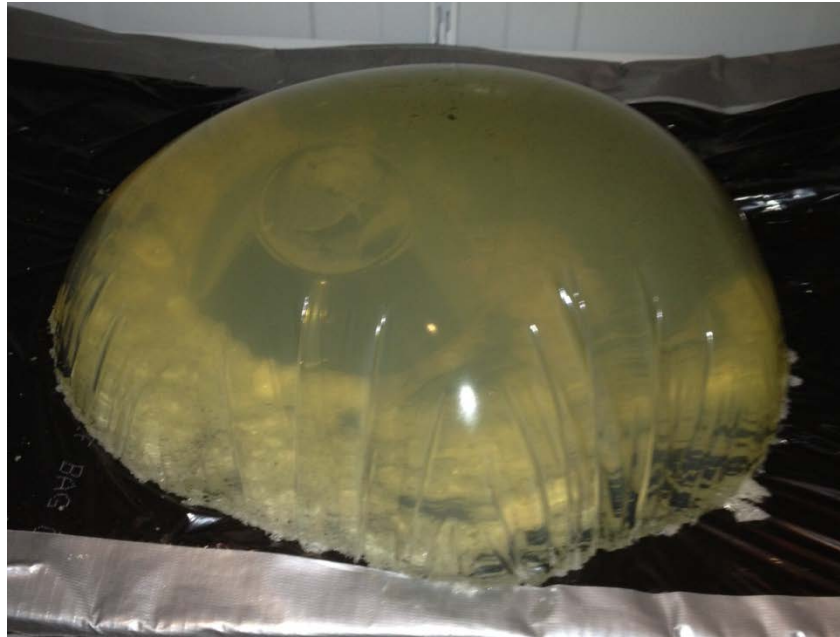
Fig. 34: Ballistics gel simulator approximating the size and shape of a maternal abdomen at full term.
