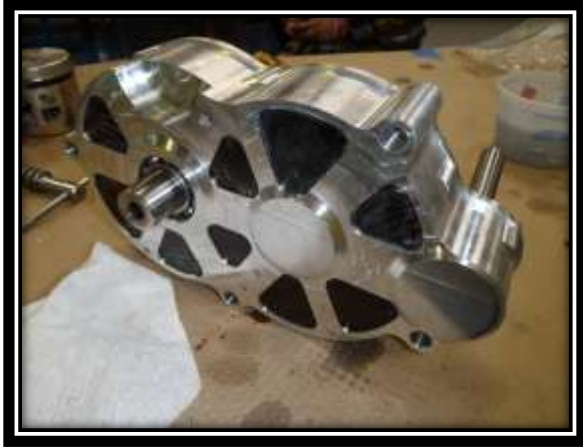
Right side of finished gearbox including carbon fiber finger guards.
