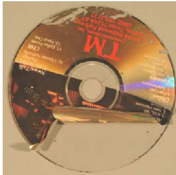
Delamination on a CD 35
