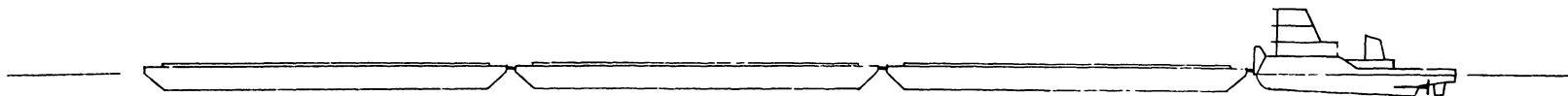
Fig. 9. Barge flotilla/towboat combination with flexible couplings. With double jumbo units operating at a draft of 9 ft, a 6500 shp towboat would give 25% power margin on a 12 knot service speed; a 3300 shp boat, 10 knots.
