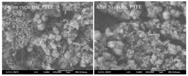
Figure S3 Morphology changes of the sulfur electrode with PTFE binder.
