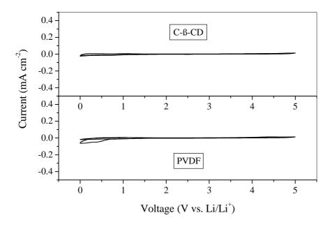
Figure S2 Cyclic voltammograms of C-β-CD and PVDF with ionic liquid of PP13 0.5M LiTFSI.
