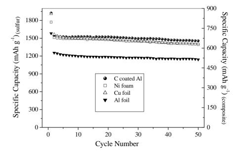
Figure S4 show the effect of current collectors including Ni foam, Cu and Al foils.
