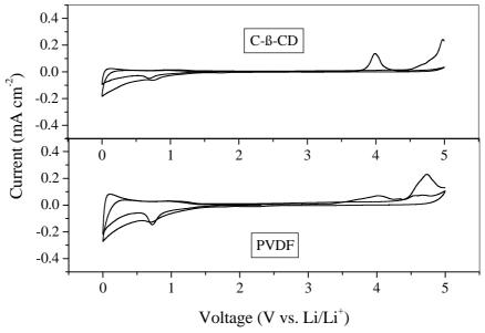
**Figure S1** Cyclic voltammograms of C-β-CD and PVDF using EC/DMC 1M LiPF<sub>6</sub> as electrolyte.
