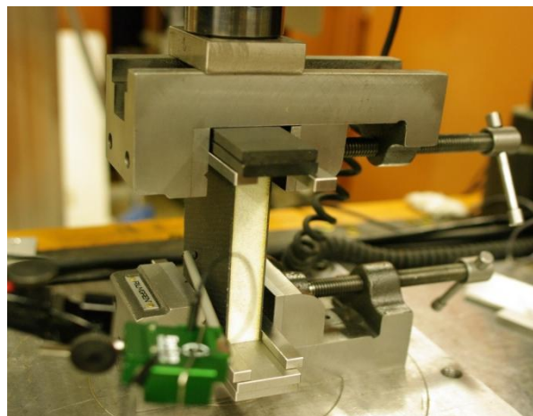
Figure 3. Edgewise compression test fixture.
