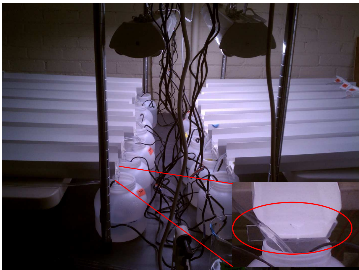
Figure 2: Photograph of the flume setup used to expose periphyton to gold nanomaterials. Inset shows a zoom of the notched dam retaining water in the channel.
