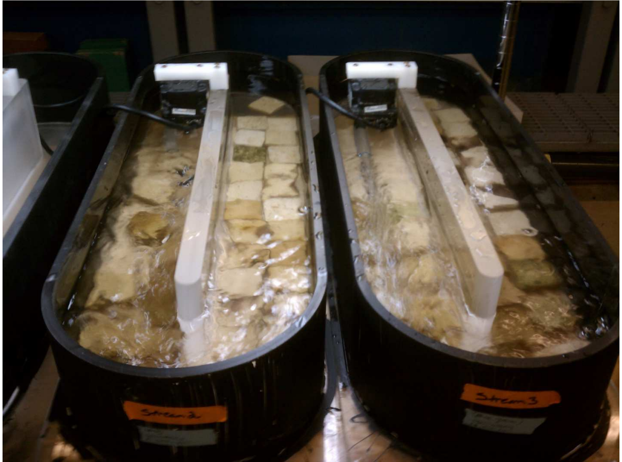
Figure 3: Image of the unglazed tiles in colonization streams during the 4-week colonization period
