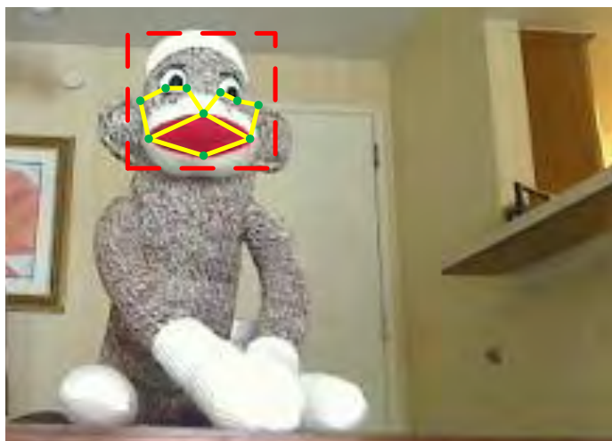
Figure 6.1 Computer Vision Example The figure shows a sock monkey sitting on a table. A computer vision application might be designed to recognize particulars in this image such as the face of the monkey. The algorithm would look for features such as corners, and use their geometric relationship to locate the monkey's face.
