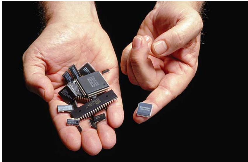
Figure 1-2 System on Chip (SoC) technology combines multiple chips into one chip.
