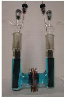
Figure 2.1.2-1 Photograph of an H-type charge/discharge cell. The blue liquid represents the volume filled with liquid electrolyte.
