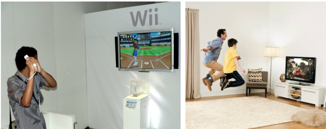
Figure 2.5. Wii provides a control to detect motion (left) and Kinect uses has a camera sensor (right;
