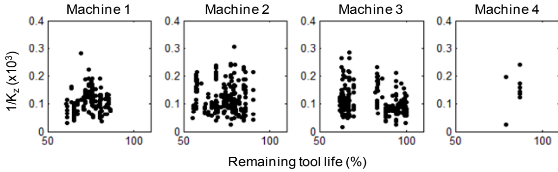
a) Stiffness of machines in Z direction
