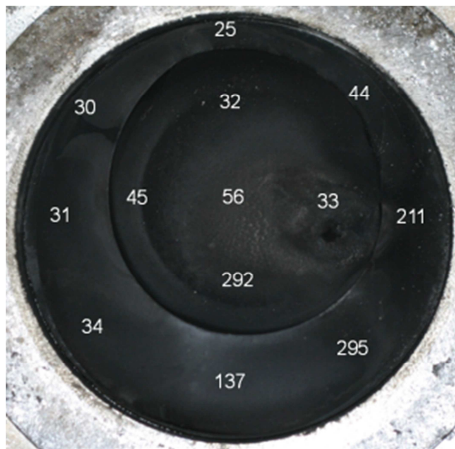
Figure 11.2 - CCD layer formed by CARBOB+10%EtOH on the piston; measurements given in \mu\text{m}
