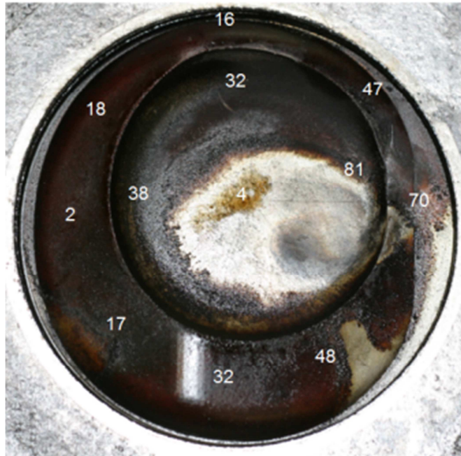
Figure 12.4 - CARBOB+10%EtOH+PEA piston deposits at the equilibrium thickness
