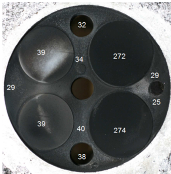
Figure 12.6 - CARBOB+10%EtOH+PBA cylinder head deposits at the equilibrium thickness
