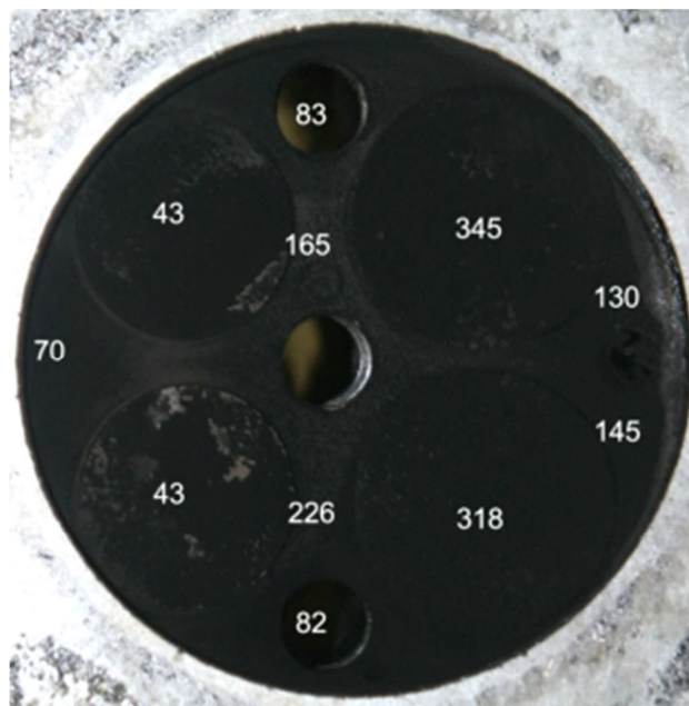
Figure 11.3. Deposit layer on the cylinder head resulting from the D10 fuel; measurements given in \mu\text{m}
