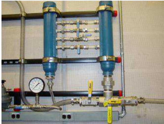
Figure 2.6 - Critical flow orifice system comprised of the orifices of known diameter to the left of the ball valves, and two manifolds to dampen any effects of pressure changes in the shop air
