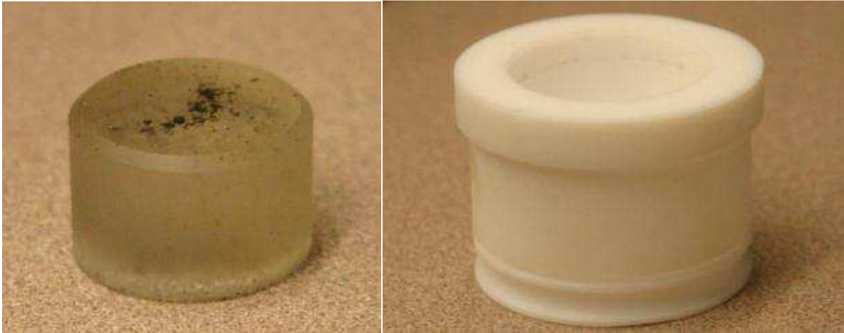
Figure 3.11 - Engine deposits cold-mounted in epoxy and molding cup used for the mounting process
