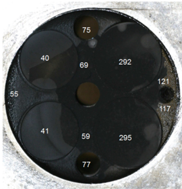
Figure 12.5 - D10+10%EtOH+PBA cylinder head CCD layer at the equilibrium thickness
