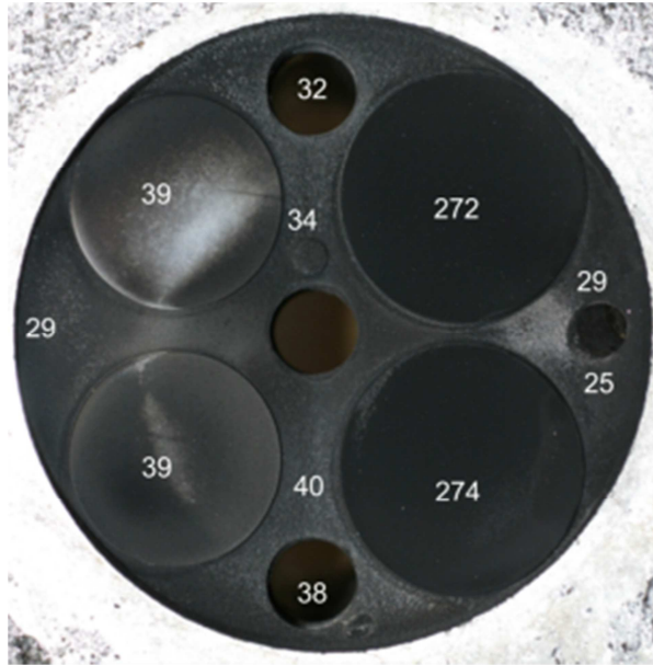
Figure 11.4 - CCD layer on the cylinder head resulting from CARBOB+10%EtOH; measurements given in \mu\text{m}
