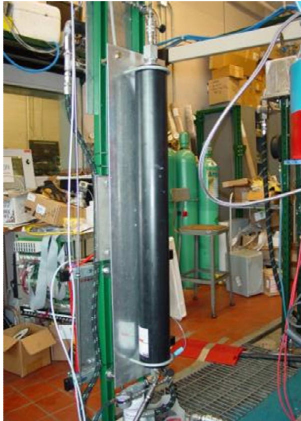
Figure 2.9 - Piston-style accumulator used to pressurize the fuel for direct injection
