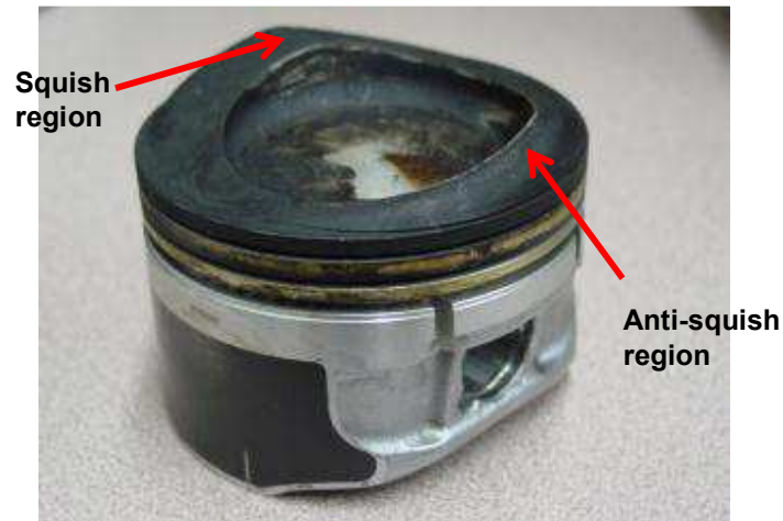
Figure 2.4 - The piston used in the single-cylinder GM HCCI fuels engine; this particular piston has a buildup of deposition clearly shown, with a notable clean spot centrally located where the fuel spray impinges upon the piston crown
