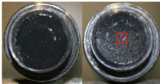
Figure 11.15 - D10 heat flux probes after engine disassembly from the fully-conditioned state; the probe from the “squish” region is on the left and the probe from the “anti-squish” region is on the right; the thermocouple junction partly visible is highlighted by the box in the picture
