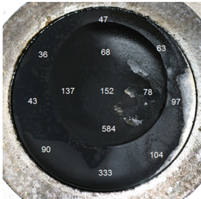
Figure 12.1 - Deposits on the piston after a conditioning sweep with D10+PBA fuel
