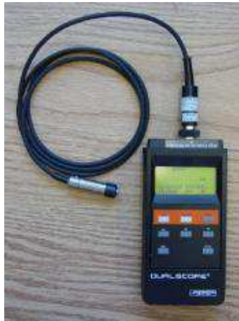
Figure 3.2 - Fischer Dualscope instrument used to measure the thickness of a layer over a substrate material
