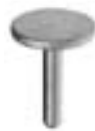
Figure 3.6 – Standard Electron Microscope (SEM) mounting stub; samples are attached to this specimen pin, and loaded into the vacuum chamber
