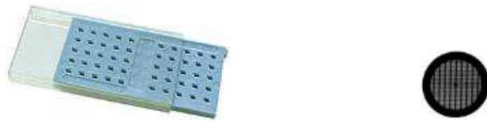
Figure 3.7 – Transmission Electron Microscope (TEM) grid storage device shown on the left with an individual grid for TEM study on the right
