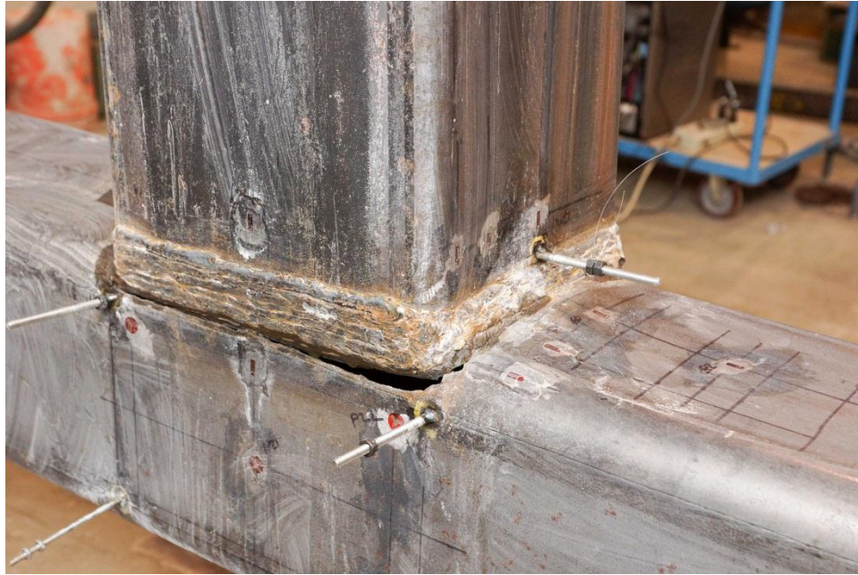
Figure 7.17 Extent of the observed fracture in the matched connection at the completion of the test.
