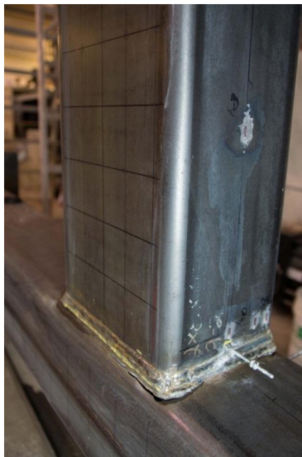
Figure 7.14 Extent of the observed fracture in the unmatched connection at the completion of the test
