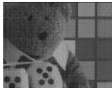
(b) Image from high-sensitivity mode (1.8V, 15 fps, 0.4 lx)
