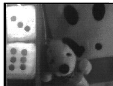
(d) Image from WDR mode (merged with different integration time: T_{INT2} = T_{INT1}/16 , 1.8V, 15 fps)
