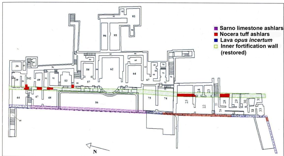
Figure 67. Pompeii, VII.16.17-22: Casa di Fabio Rufo and Casa di Maio Castricio, plan of basement indicating the location of the original fortification wall (after Cassetta and Costantino 2008).
