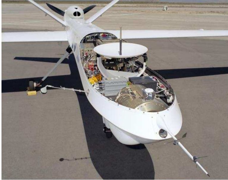
Figure 1.1: UAV with top panel removed showing bulky gimbal-based antenna steering mechanism [1].
