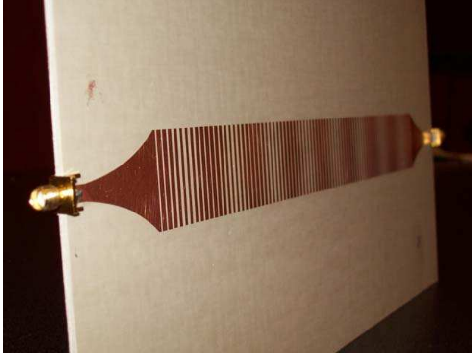
Figure 2.14: Photograph of fabricated antenna with a 50\Omega termination at one end.
