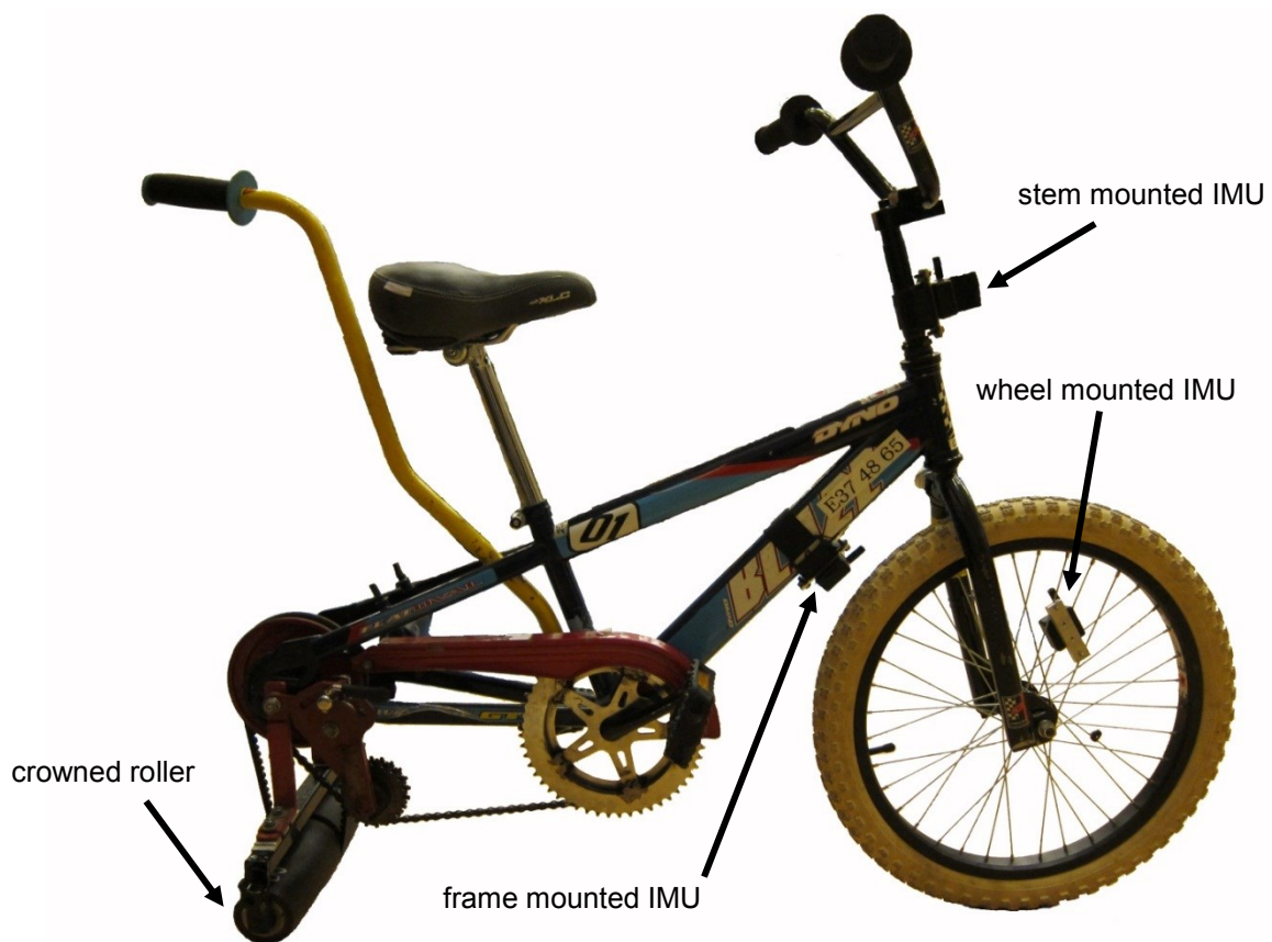
Figure 4.1. An adapted bicycle. The adapted bicycles used by Lose the Training Wheels utilize crowned rollers in place of a rear wheel. The roller is driven by a belt, which is driven by a pulley connected to a standard bicycle transmission. In addition, the bicycles also have a handle attached to the rear of the bicycle that allows a trainer to assist the rider as needed. For this study, three wireless inertial measurement units (IMUs) were mounted the bicycles: one on the frame (frame mounted IMU), another on the handlebar stem (stem mounted IMU), and one on the spokes of the front wheel (wheel mounted IMU).
