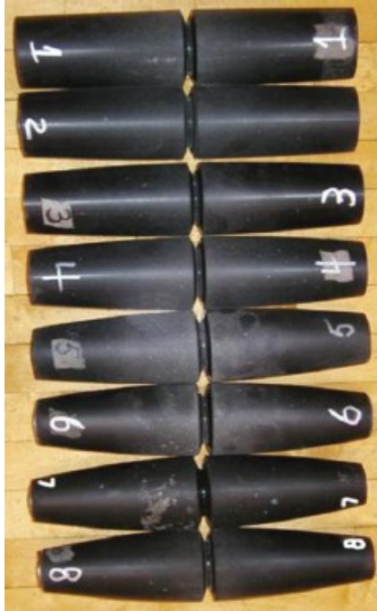
Figure 4.2. The rollers used on the adapted bicycles. A series of crowned rollers is used to modify the characteristics of the adapted bicycle. Roller number 1 (top) has the smallest crown (less lean/greater stability) while roller number 8 (bottom) has the largest crown (most lean/least stability). Participants often begin with roller number 3 and end with roller number 6 before advancing to a traditional bicycle.
