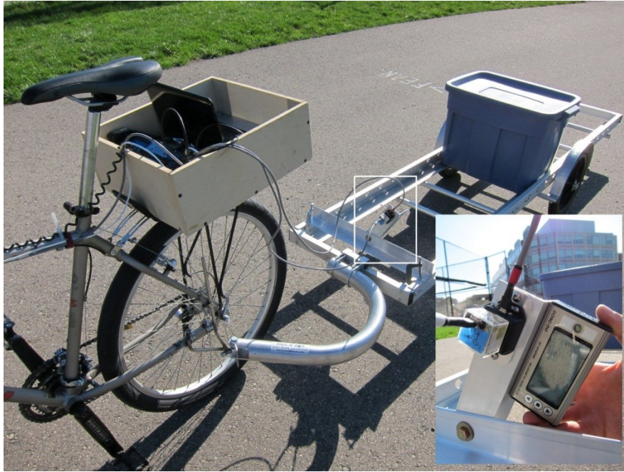
Figure 3.3. A jig was used to validate our method of estimating the bicycle roll angle by allowing us to orient the inertial measurement (IMU) at a fixed simulated roll angle. The simulated roll angle was independently measured using an inclinometer that can resolve the roll angle to within \pm 0.01 degrees (inset photograph). The jig was secured to a bicycle trailer and pulled behind the instrumented bicycle on level pavement. The white rectangle indicates the location of the IMU on the jig secured to the trailer.
