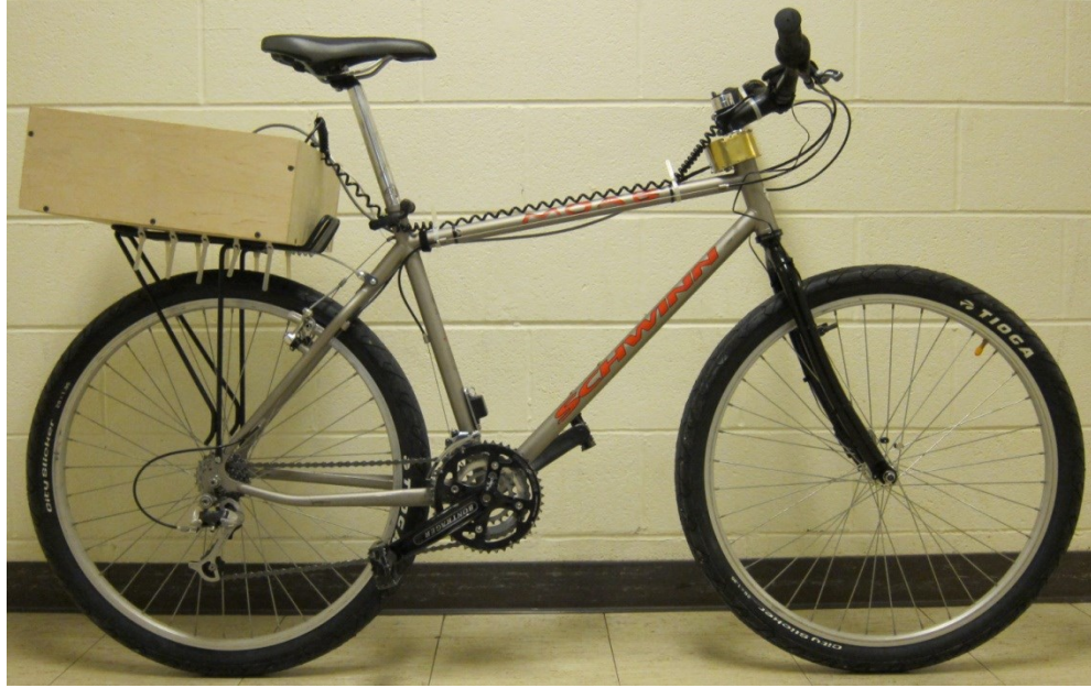
Figure 2.1. The instrumented bicycle. The instrumented bicycle is a standard geometry mountain bike equipped to measure: steering torque, steering angle, bicycle speed, bicycle angular velocity about three axes, and acceleration along three axes. A laptop computer, A/D boards, battery, and circuitry are supported in a box at the rear.
