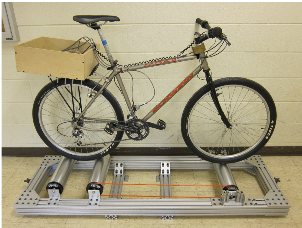
Figure 5.9. A photograph of the instrumented bicycle on the custom rollers. Note that the bicycle is leaning against the wall to stay upright.
