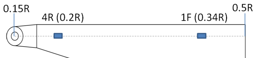
Figure D-12: Location of Strain Gages used for the Pull Test of Root Section
