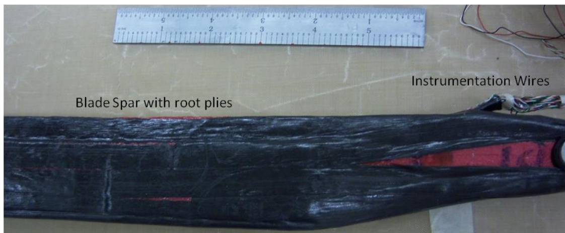
Figure E-22: All Root Plies wrapped around the Root Pin
