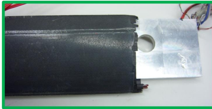
Figure E-60: Fabricated Section for Pull Test
