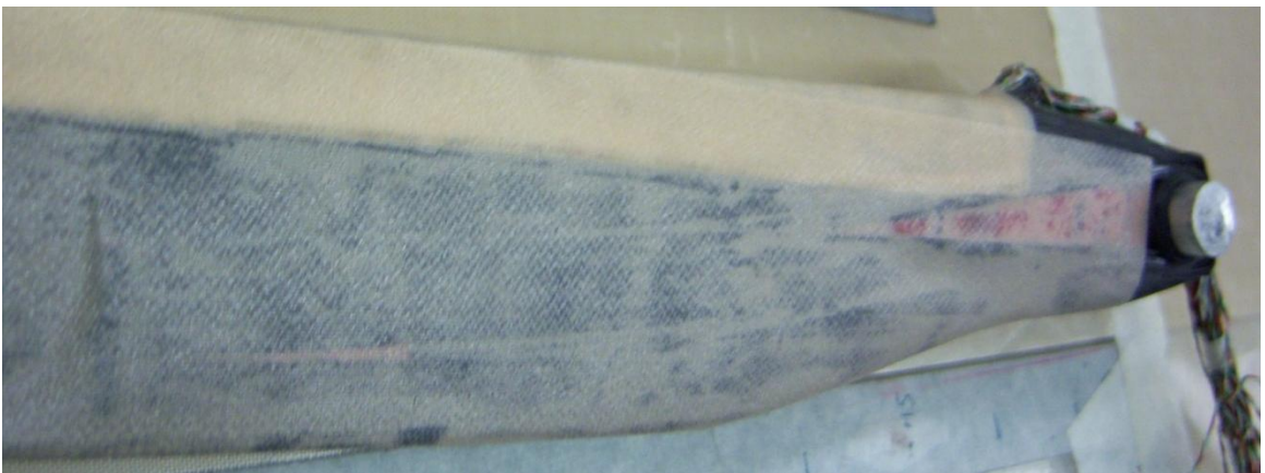
Figure E-26: First Main Spar Ply near the Root Region
