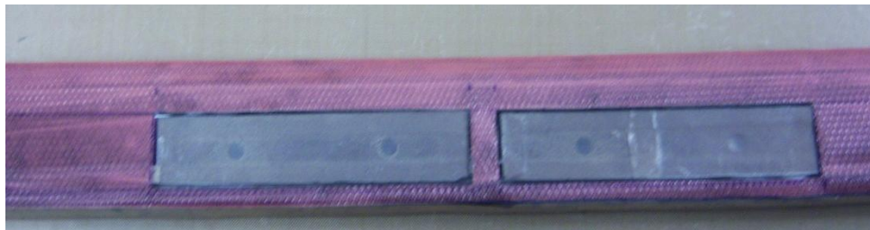
Figure E-29: Cutout Region with All Spar Plies
