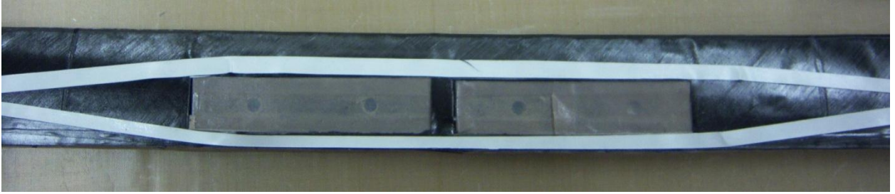
Figure E-28: Unidirectional Plies moved around the Cutout Region
