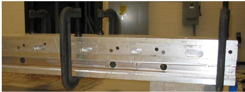
Figure E-34: Blade Molds Closed with Heavy Duty Steel Clamps
