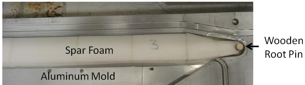
Figure E-4: Joined pieces of Foam Core
