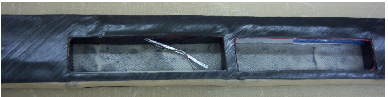
Figure E-27: 4th Spar Ply in the Cutout Region
