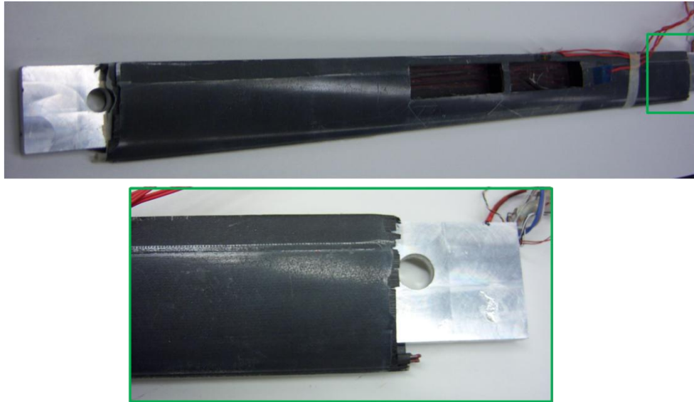
Figure D-16: Test Section Fabricated for Pull Test of Cutout Section
