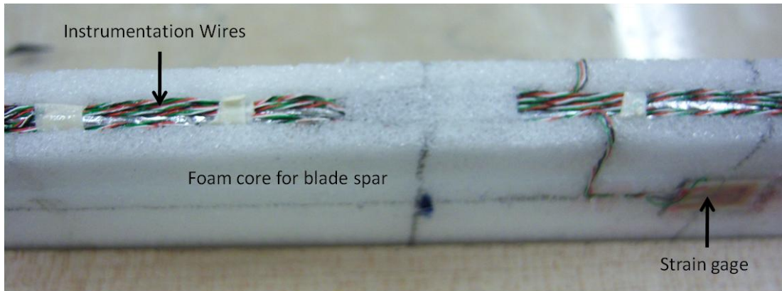
Figure E-7: Trough made in the Blade Spar for Instrumentation Wires
