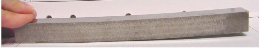
Figure 4.9. Bowing of a bar due to the roll burnishing.
