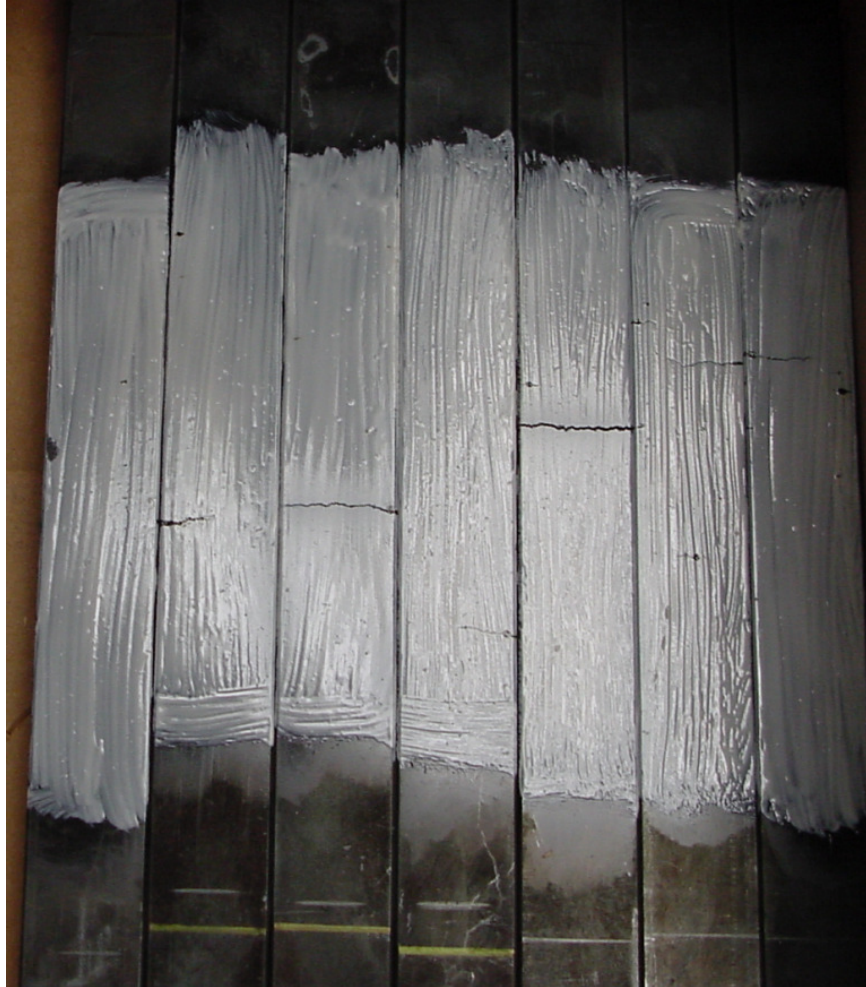
Figure 4.7. Stress-relieved LRB samples after fatigue tests with applications of ZnO paste.
