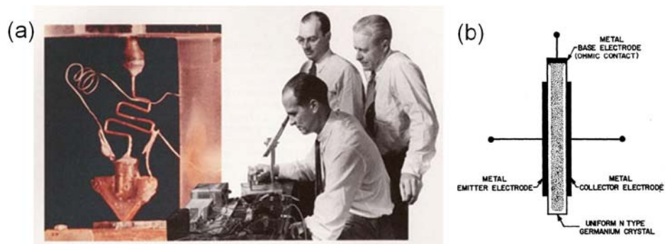
Figure 5.3 (a) The very first transistor ("point contact transistor") invented by William Shockley, John Bardeen, and Walter Brattain in 1947. (b) The structure of the surface barrier transistor (adopted from [135])
