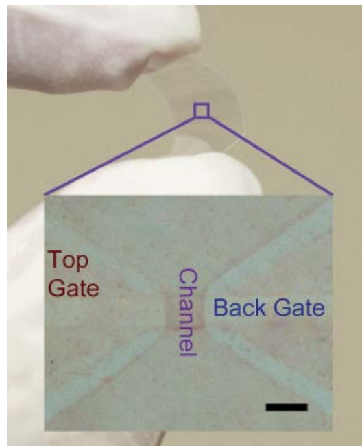
Figure 4.7 a photograph of graphene circuit on a transparent and bendable plastic substrate, and a microscopic image of an all-graphene transistor (inset). The scale bar is 10\mu\text{m} .
