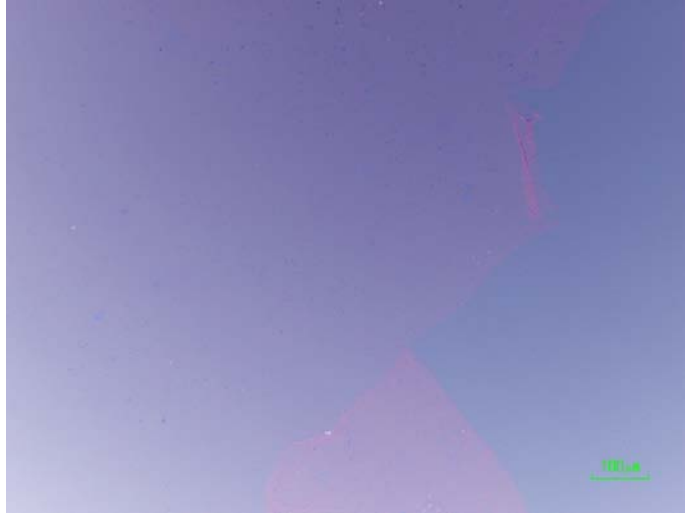
Figure 2.3 Optical microscopy image showing the edge of bilayer graphene film. Scale bar is 100 \mu\text{m} .
