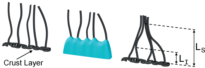
FIG. 3. (Color online) One-dimensional schematic of CNT self-assembly due to elastocapillary aggregation.
