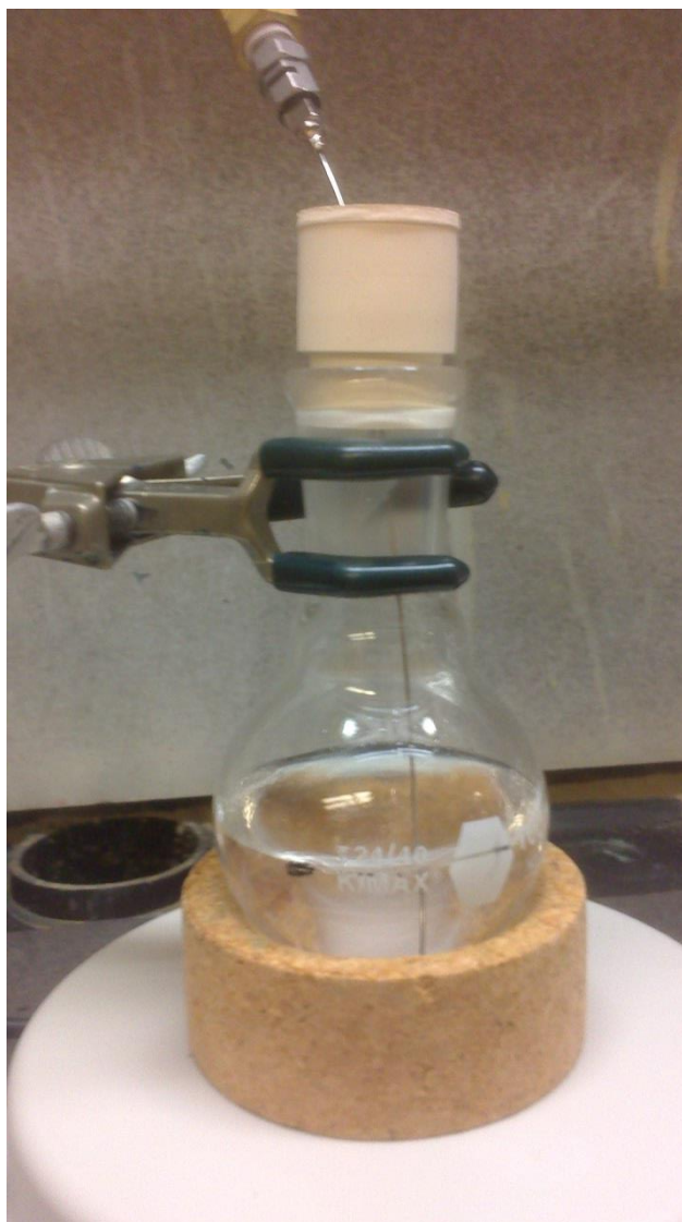
Figure 12: Reverse micelle polymerization reaction setup containing hexane and aqueous phase stirring under an argon atmosphere.
