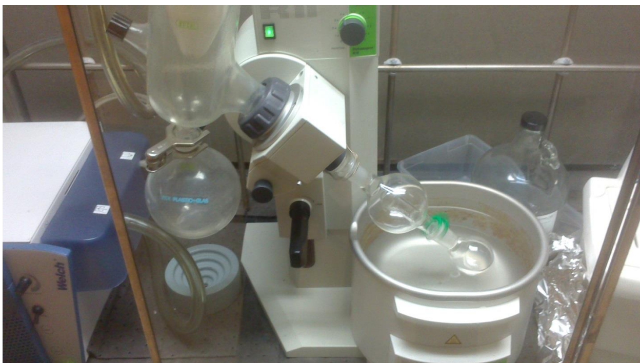
Figure 13: Rotary evaporation of polymerized nanoparticle reaction flask. The solution becomes milky white and viscous as hexane is pulled out of the mixture.
