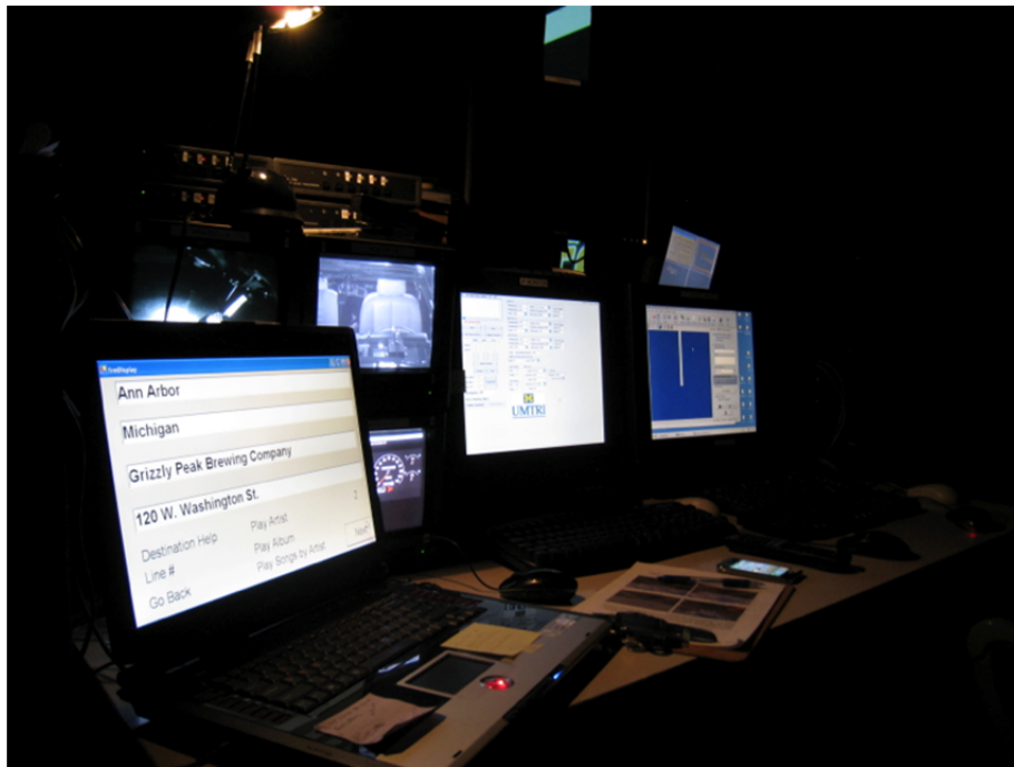
Figure 4-2. Simulator Operator's Workstation
