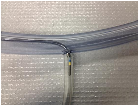
Fig. 3.7. Tygon tube model used to test that the final catheter is able to make the bend and get to the renal artery. The aorta and renal artery diameters are assumed to be 1 cm and 0.5 mm respectively.
