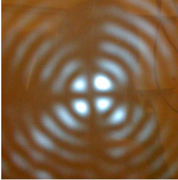
Figure 3.6: An example of a Maltese cross pattern formed by a cross polarization setup and a high NA objective. Photo courtesy of Jieun Lee.
