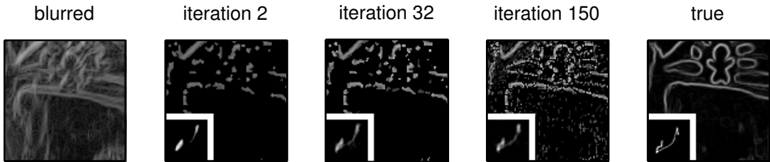
Figure 3.1: Kernel estimation on an image from the test set of [71]; a small patch has been selected and rescaled for clarity. Left: Blurry edge map |\mathbf{y}| . Center left to center right: Evolution of the kernel k (inset) and edge map magnitude |\mathbf{x}| in the final full-resolution stage. As \tau increases in (3.6), the edge map becomes less sparse and the kernel is refined. Right: k^{\text{true}} and |\mathbf{x}^{\text{true}}| .
