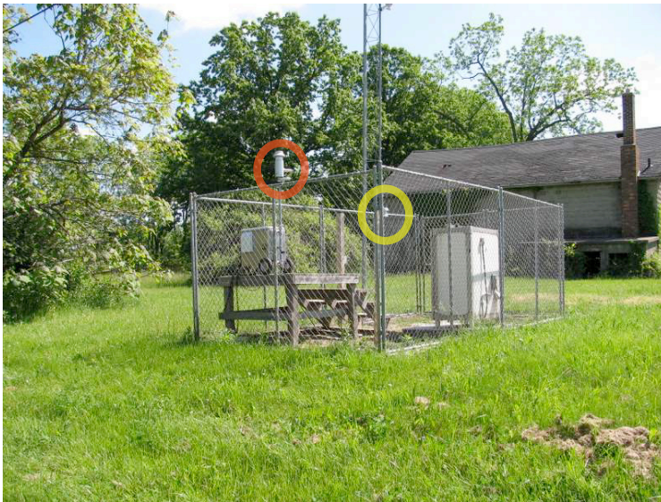
Figure 4.4: A photograph taken of the Joy road observing site. This location was a site of MDEQ and HOBO co-location. The MDEQ monitor is circled in red and the HOBO monitor circled in yellow.
