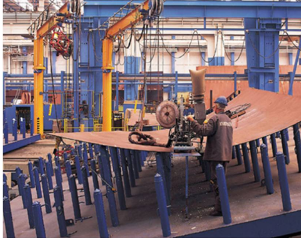
Figure 2.2: Curved Panel Assembly Line
