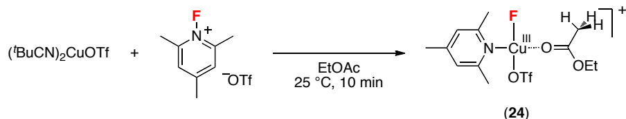
Scheme 5.5. Reaction of ( t BuCN) 2 CuOTf with NFTPT in Ethyl Acetate
