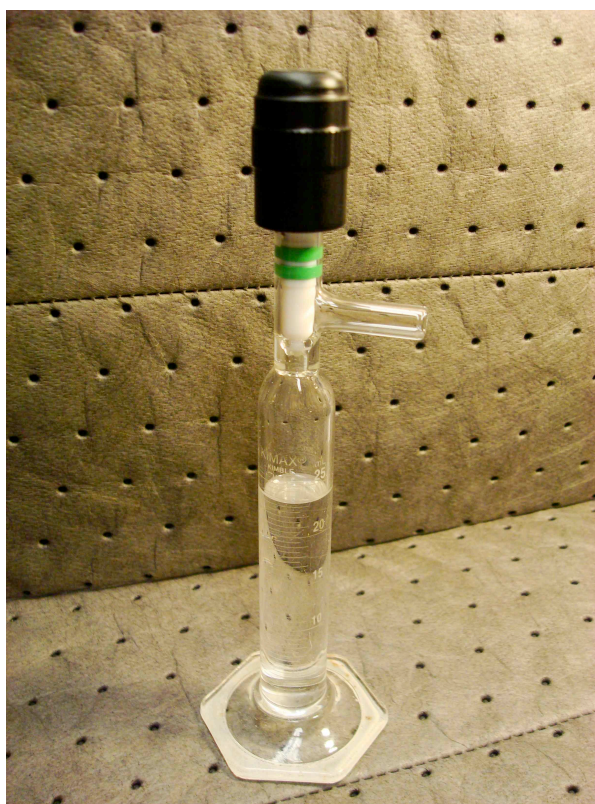
Figure 2.1. Schlenk Graduated Cylinder with CF 3 I Stock Solution
