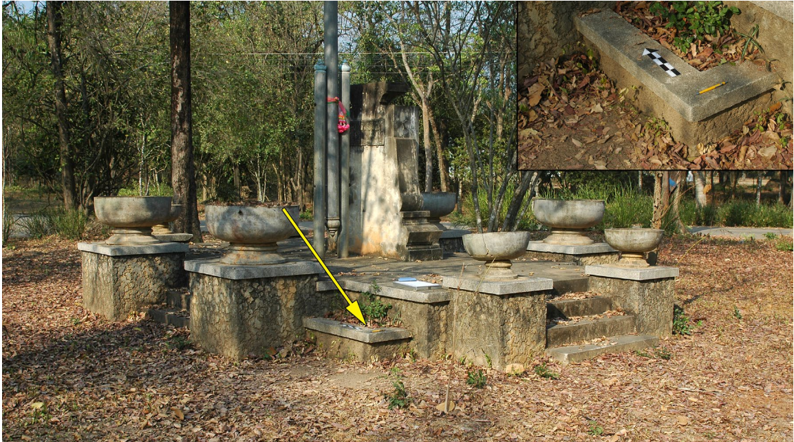
Figure D.2. Location of the datum point on the southwest corner of the flagpole monument at the center of Kamphaeng Saen (view northeast). In the inset photo the tip of the pencil is at the datum point.
