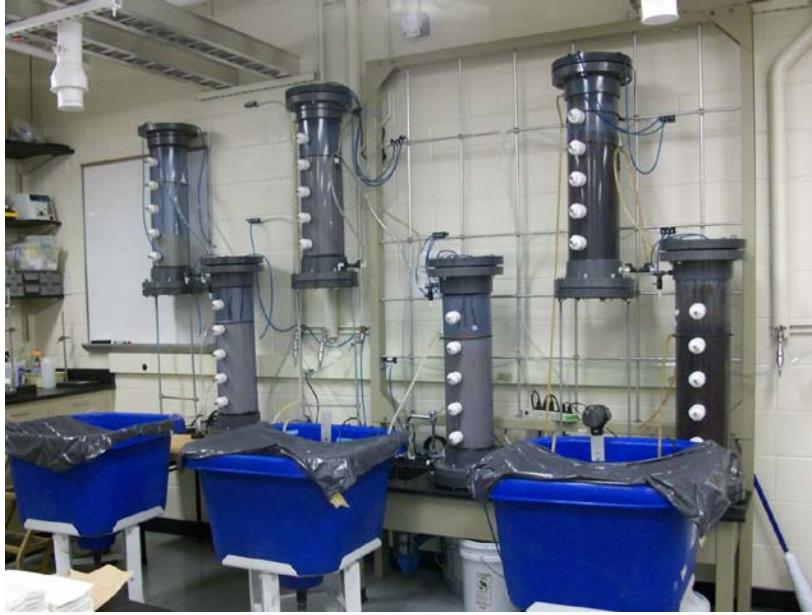
Figure 4.1. Three replicate RAS. Each reactor consisted of a culture tank and two biological aerated filters. Water was pumped from the tank to the first filter and then flowed by gravity through the biofilters back to the tank.
