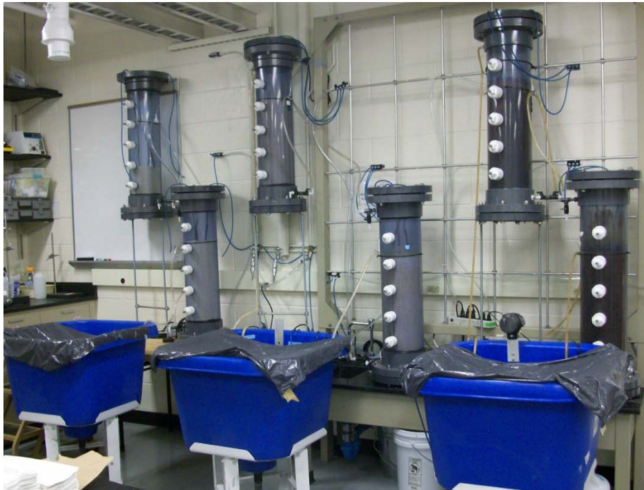
Figure A2.1: Three RAS reactors
