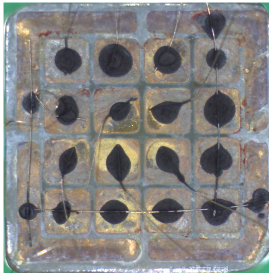
Figure 6.18: Optical microscope images of the anode of detectors 70BA1L after failure. The bottom row and right column of pixels are connected and serve as a guard ring. The anode pixels are oriented such that pixels 1, 2, and 3 are in the top row. Large portions of the gold contact are missing in this detector
