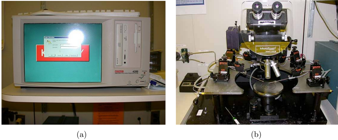
Figure 7.11: (a) Keithley 4200 semiconductor characterization system and (b) the Alessi probe station used to measure HgS I-V characteristics. The device being tested was placed on the probe station stage, and the probes were put in contact with the electrodes. Then the probe station is connected to the Keithley which controls the voltage and measures the characteristics.
