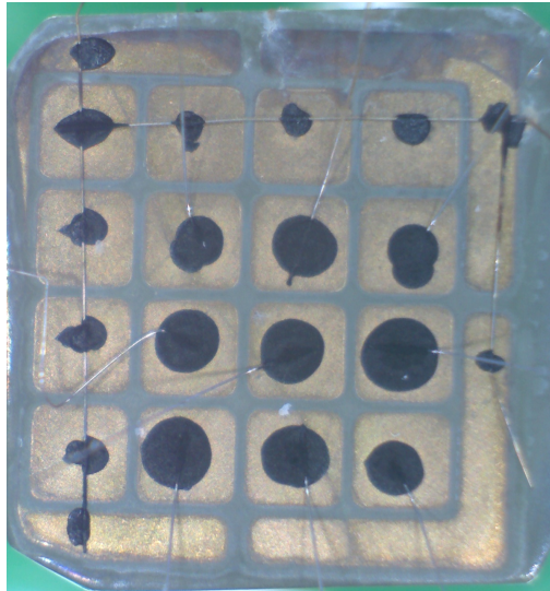
Figure 6.17: Optical microscope images of the anode of detectors 70BA1R after failure. The top row and left column of pixels comprise the guard ring, and the anode pixels are oriented such that pixels 1, 2, and 3 are in the top row. Any physical damage to the contact is not visually obvious.
