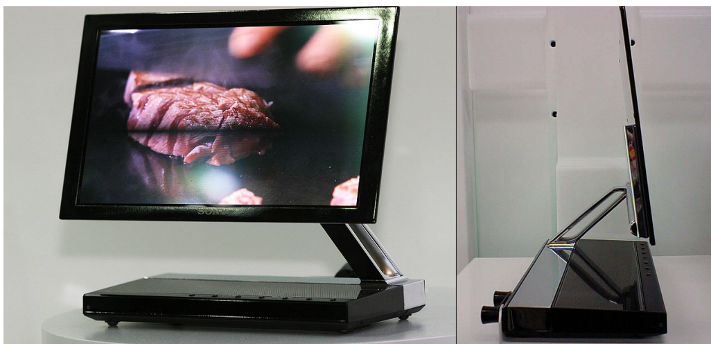
Figure 2.1 The world's first OLED television, featuring a 3 mm thick display. Courtesy of Wikimedia commons.
