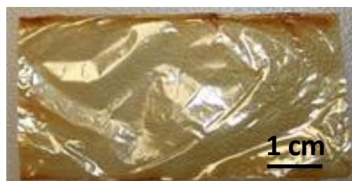
Figure 3.3 An ANF film made by layer-by-layer assembly showing uniformity and transparency.
