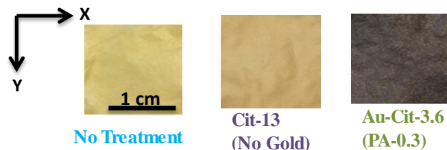
Figure 7.1 Optical micrographs of three aramid network samples showing the change of color through the addition of gold nanoparticles. The samples change from transparent and yellow (“No Treatment”), to translucent and yellow (“Cit-13” with PA and citrate treatment), to translucent and purple (“Au-Cit-3.6” with PA, citrate and AuNPs). The isotropy of the samples was checked by testing specimens at different orientations in the X-Y plane and from nano-indentation testing on the thickness direction [4].
