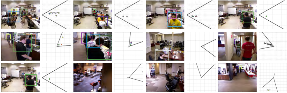
Figure 2.12: Examples of tracking results. First row: results on the Kinect office dataset . Second row: results on the Kinect mobile dataset . Detections are shown as boxes in images, and dots projected onto the ground plane in the top-down view. Each color is a person. Note that our system detects people in various poses, truncated by the image, and despite the severe occlusions between people that are common in indoor environments. The last row shows examples of challenging scenes where the people appear beyond the Kinect’s range or under extreme lighting conditions.
