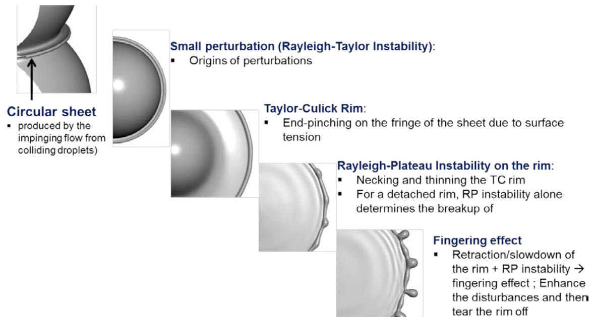
Figure 5-20. Interface evolution: instabilities on the edge of the circular sheet.
