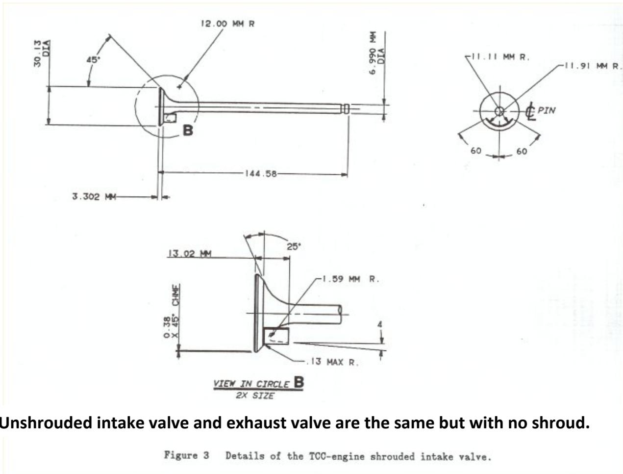
Unshrouded intake valve and exhaust valve are the same but with no shroud.
