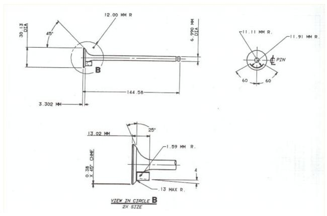
Unshrouded intake valve and exhaust valve are the same but with no shroud.
